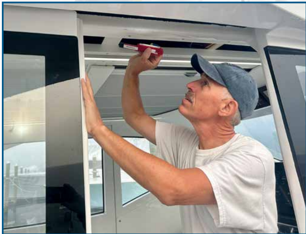
Charlie Munro, who specializes in exterior fit and finish, uses an LED inspection light to check the frame of the powered pilothouse side door on a 55 Sport Yacht.
